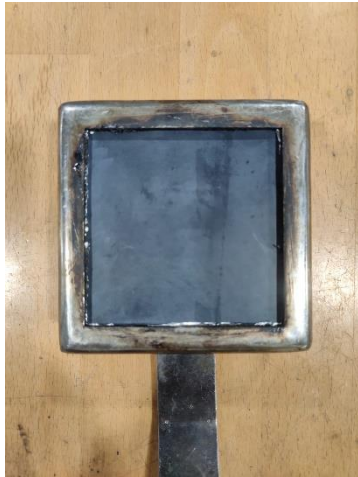
Sample Before Test (ISO 5659-2)
