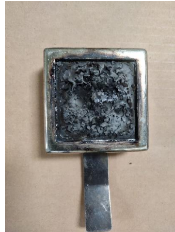
Sample After Test (ISO 5659-2)
